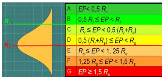
Figure 1 Energy performance Rating - example
